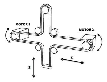
The 2 motors should turn at the same time and against each other depending on the requested movement of the Axis.
