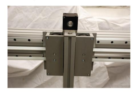
In 2014 and 2015 several of these systems have been built for other applications; And with a 40x40 profile in the Z-axis instead of the original 40x80
