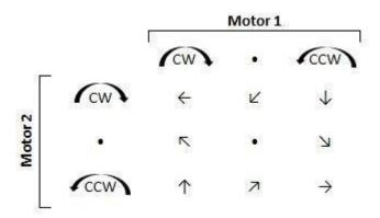
If both motors are powered at the same time it gives the maximum acceleration (deceleration).
